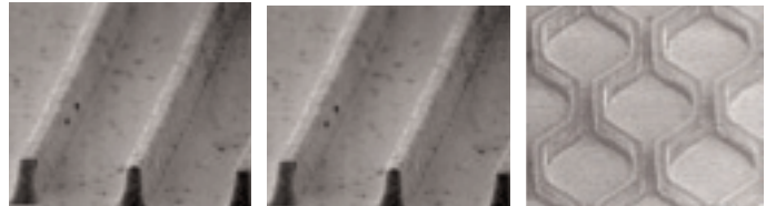
Examples of the barriers that isolate each cell. The distance between the walls of each cell is a couple hundred micrometers – or about ten times the diameter of a human hair.
