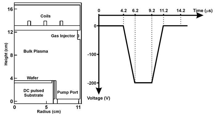
Fig. 1. Schematic of the reactor and pulsed bias voltage waveform.
