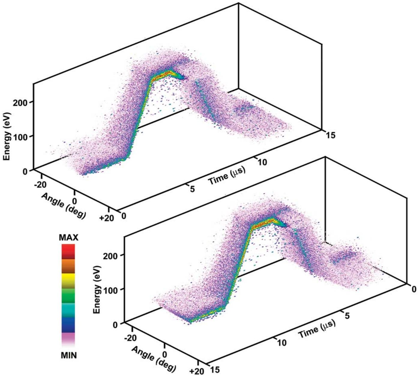
Fig. 2. Time evolution of the IEAD in an ICP with a pulsed dc bias on the substrate. Views are shown from the perspective of early and late times, with cutouts to reveal the high intensity portions of the IEAD. IEAD narrows as the bias voltage decreases to its most negative value.
