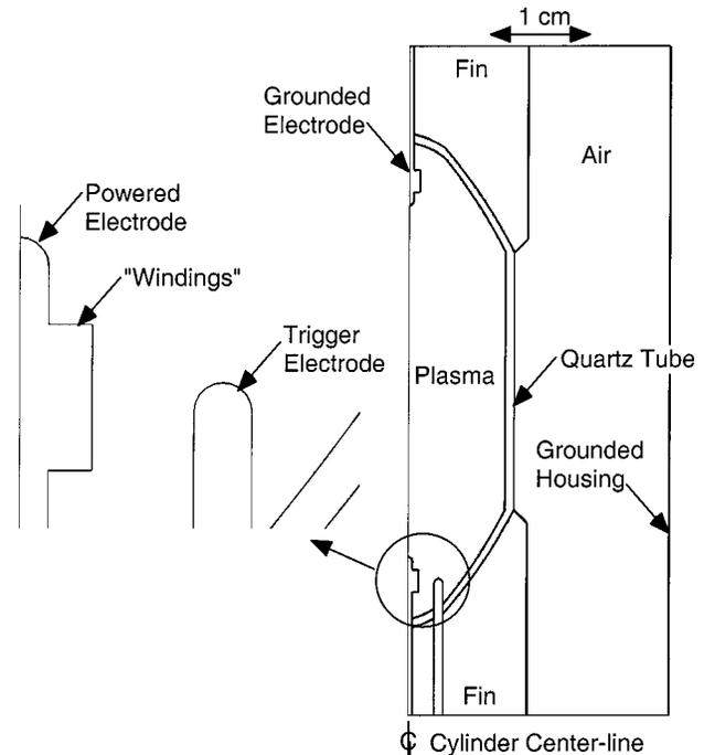
Fig. 1. Schematic of the cylindrical model lamp geometry.
