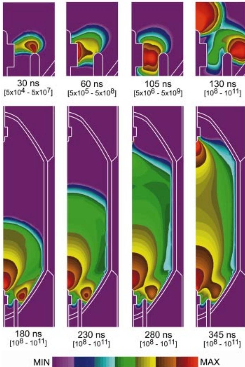
Fig. 2. Electron density at different times during gap closure as noted below each figure. The range ( $\text{cm}^{-3}$ ) of the electron density in the figure is noted in the brackets. The trigger pulse ends at 90 ns. The sustain pulse begins at 115 ns and ends at 400 ns.
