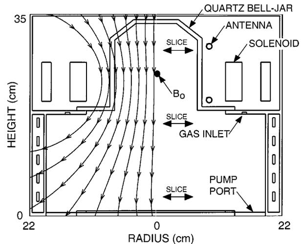
Fig. 1. Schematic of the squat helicon reactor. The streamlines show the magnetic field (azimuthally symmetric), 100 G at  $B_0$ . The double arrows show the heights of the axial slices in Fig. 2.
