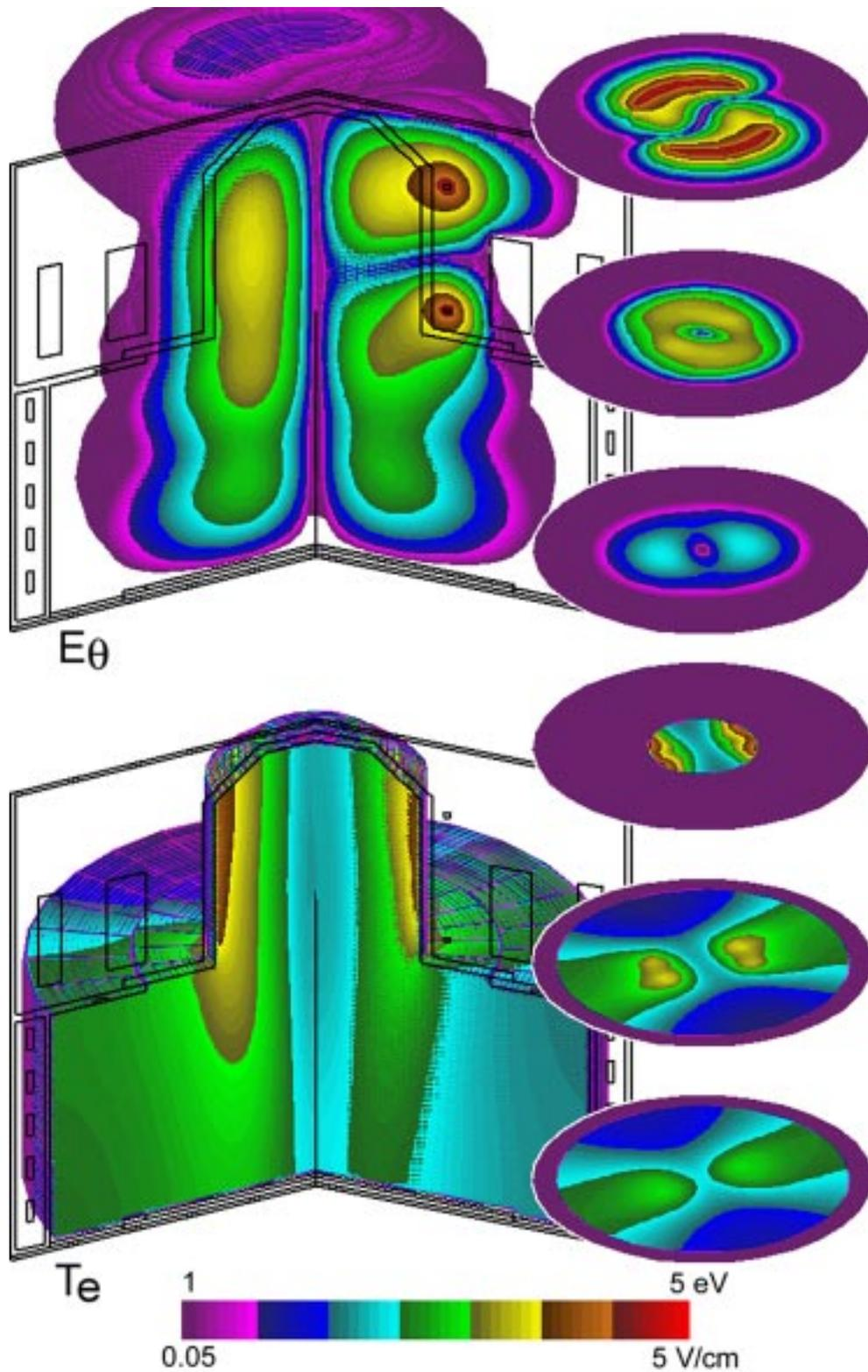
Fig. 2. Azimuthal electric field (top) and electron temperature (bottom). The radial slices through the 3-D images are through the antenna (right) and through the gap in the coils (left). The axial slices are at the heights noted in Fig. 1.
