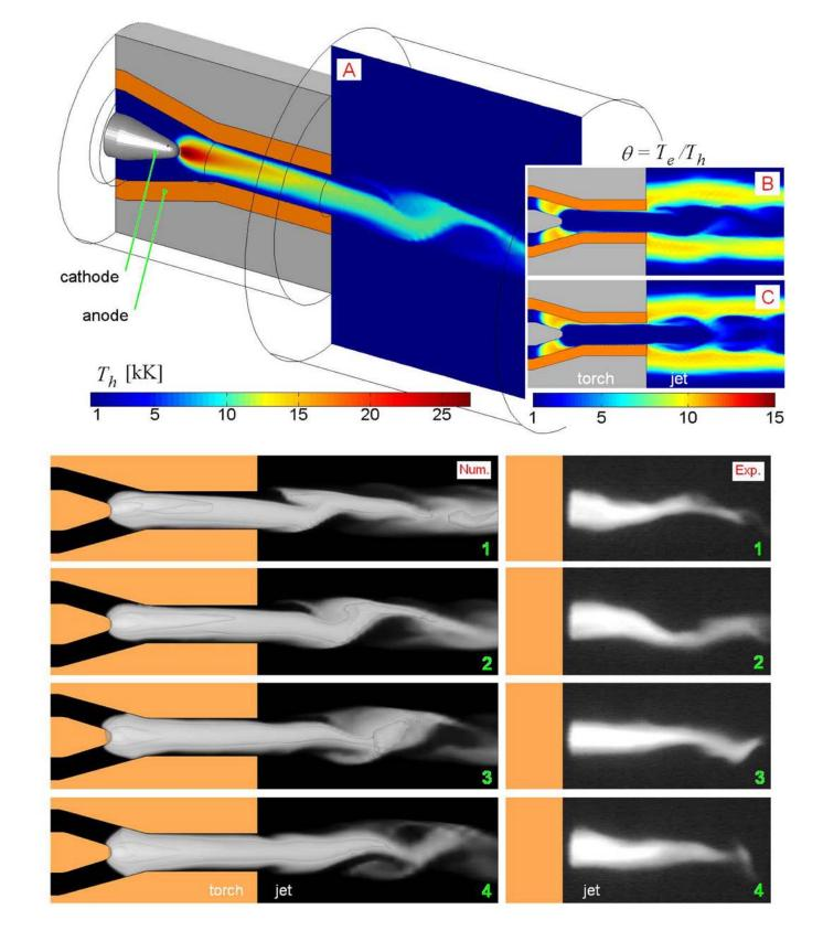
Arc Plasma Jet (top) Calculated heavy particle temperatures (Ar, 400A) (bottom) Model and experiment of plasma emission.
